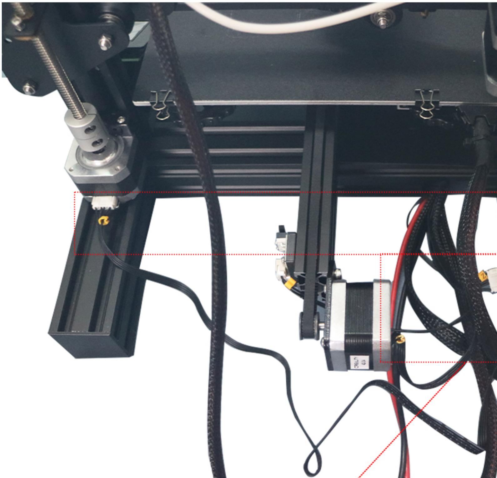
Connect the stepper cable of motor
