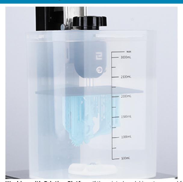
**Washing with Printing Platfrom** If the printed model is not removed from the build platform, please mount the build platform to the adjustable platform bracket (The height of the platform bracket can be adjusted to fit the liquid level in the bucket, up to a maximum model height of 120 mm), then hang the adjustable platform bracket on top of the pillar to start the cleaning.
