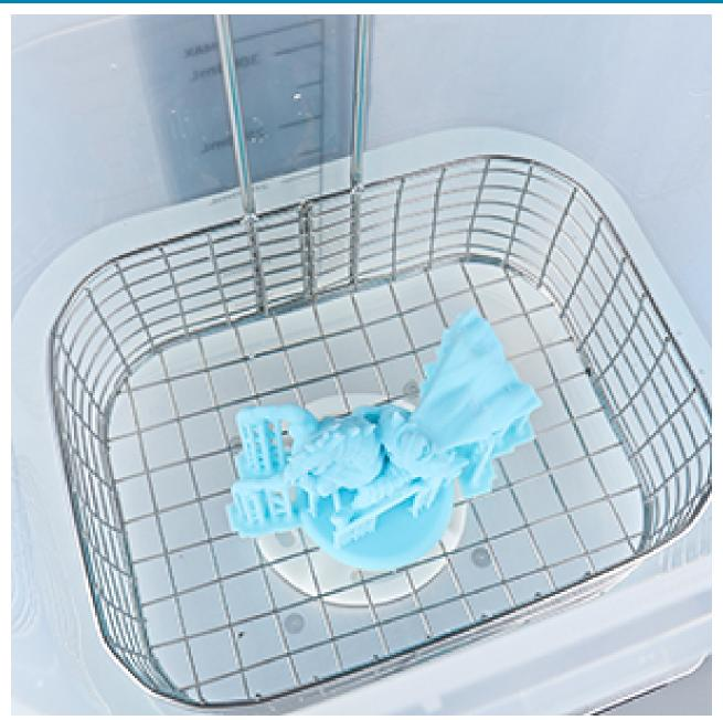
**Washing with Bucket** If the printed model has been removed from the build platform already, you will need to place the model in the cleaning basket (maximum model height is 160 mm) and hang the cleaning basket on top of the pillar to start cleaning the model. Models larger than 15 mm in size are available with this cleaning option. Some small models can be cleaned together in the bucket.
