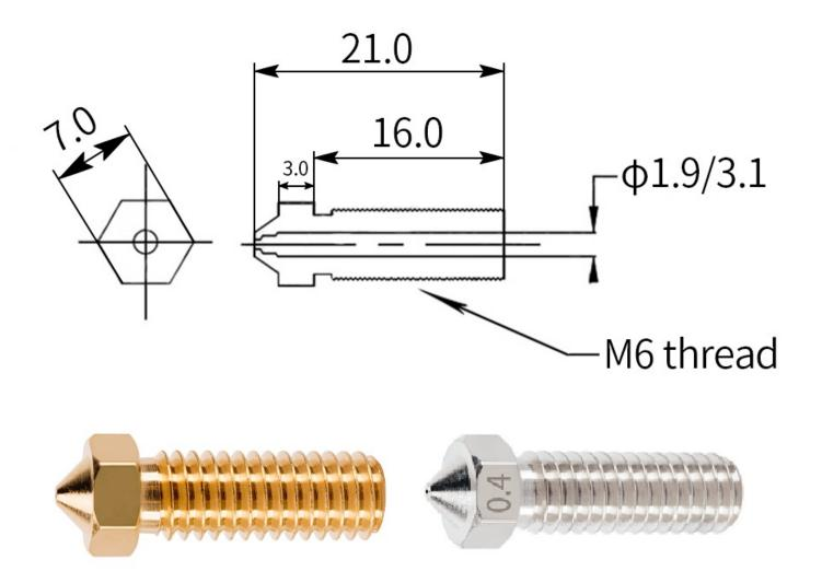
Material: brass, stainless steel Input diameter : 1.75mm/3mm Output diameter: 0.2/0.3/0.4/0.5/0.6/0.8/1.0 /1.2mm
